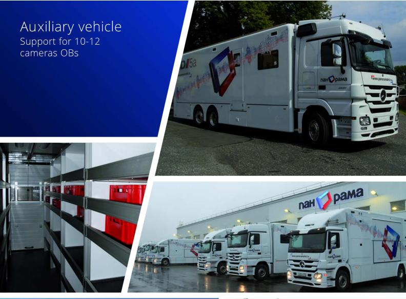
Design, System integration Construction of the van Two areas inside - Crew area, Stowage area Tail lift Air-conditioning Designed to operate in diverse climatic condition
