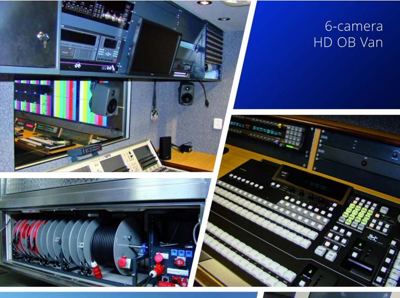
Design, System integration SONY HXC-100 cameras For-A production switcher Audio mixer Soundcraft Vi4 Harris routing Monitoring, interfacing, etc.
