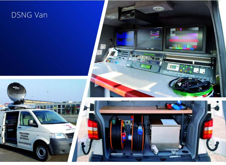
Construction of the van Fischer Panda generator - SweDish DA120-180W Antenna, Tandberg encoder SONY PDW-700 camcorders with Telecast fiber system Monitoring, interfacing, racks, furniture, etc
