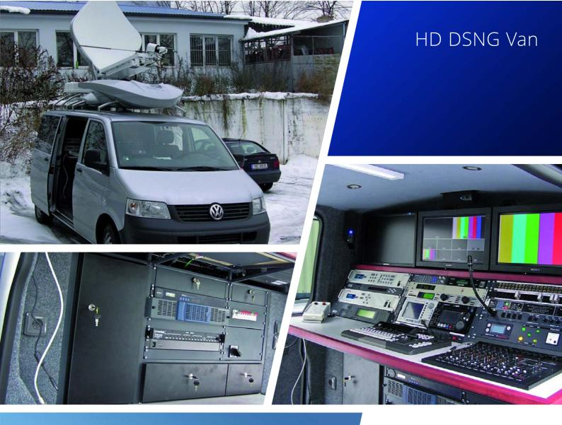
Construction of the van Fischer Panda generator ND-Sat SkyRAY Compact 1500 Antenna, Tandberg encoder SONY PDW-700 camcorders with Telecast fiber system ForA HVS-300 switcher Monitoring, interfacing, racks, furniture, etc.
