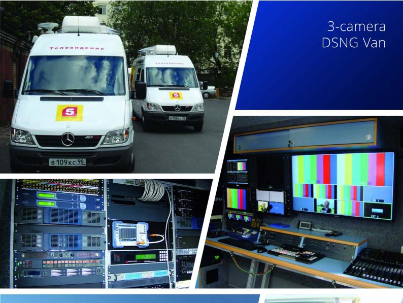
Construction of the van (single side expandable) SONY HSC-300 cameras ForA HVS300 production switcher Harris routing Satmission antenna Monitoring, interfacing, racks, furniture, etc. Designed to operate in diverse climatic conditions
